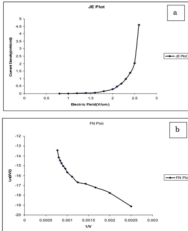
**Fig. 2** –  $JE$  plot of CNTs grown by LPCVD (a) FN plot of CNTs grown by LPCVD (b)
