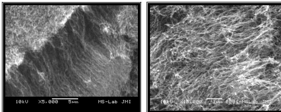
*Fig. 1 – SEM micrograph of CNTs grown by LPCVD*
